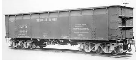
C&O 120-ton six-axle "battleship" gondola, c. 1920.
